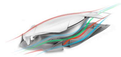
v=250 Km/h Frontal area = 1,9876m2 Cx = 0,80Aero performance = 444 Cv Cza = -0,300 - F Lift Czp = -0,300 - R Lift Fa = - 179 kg - F Downforce Fp = - 179 kg - R Downforce The name Torq derives from the huge torque transmitted to the ground by the four electric motors, which reach 1800 Nm. As a simple comparison, modern Formula One racecars have 1000 Nm of torque.
