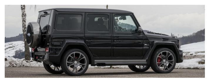
The large and wider wheel arches are filled with forged monoblock wheels in sizes of 11 x 23 inches, which are covered with 305/55 R 23 size tyres. The time-consuming production process guarantees the excellent qualities of the high-performance rims. During the forging process, the material is compressed to a point where all air inclussions are forced out of the aluminium.
