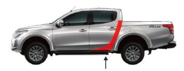
Since then, the market has changed, calling for a more substantial look. In parallel, MMC Engineering also had to work on aerodynamics - successfully with a Cd of...40 (from .46 for the previous L200) while keeping weight within reasonable limits for an excellent power/weight ratio (10.36 kg/ps\*) and optimizing space, all to support Mitsubishi's quest for fuel economy and low CO<sub>2</sub> emissions.
