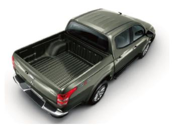
The new L200 remains within the "5 meter class" (5,205 mm for the Double Cab), helping with parking, manoeuvring (with still the tightest turning radius in its class – 5.9 m) as well as weight, the latter being a key factor for good fuel economy and therefore low  $CO_2$  emissions, all translating into low running costs for independent professionals or small businesses.
