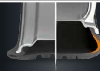
PNEU CONVENTIONNEL | PNEU DRIVEGUARD
