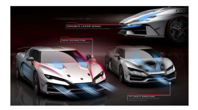
The air enters the central intake, flows along a "Y-shaped" path and emerges from the two apertures inserted in the upper part of the bonnet, thereby generating **downforce**.
