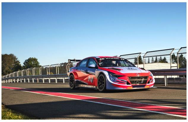
Powered for performance by a new two-liter turbocharged I-4 engine derived from Hyundai's all-new Elantra family of road-going models, the front wheel drive Elantra N TCR shares the same six-speed, paddle-shift operated gearbox as the proven Veloster N TCR and the i30 N TCR.
