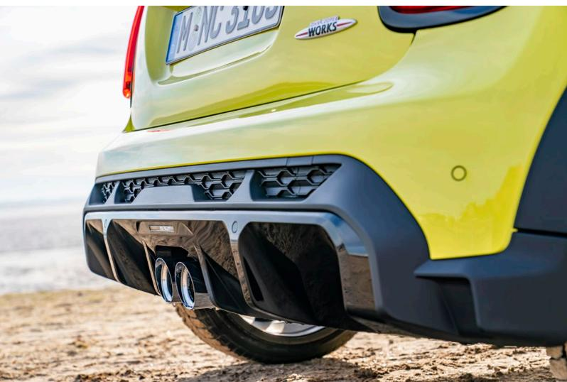
The Union Jack design rear lights are a subtle reminder of the brand's British origins. And the powerful contours of the rear diffuser, in the centre of which the two 85-millimetre stainless steel tailpipes of the exhaust system protrude into the open air, also signal authentic sportiness. This also applies to the sound of the sports exhaust system,
